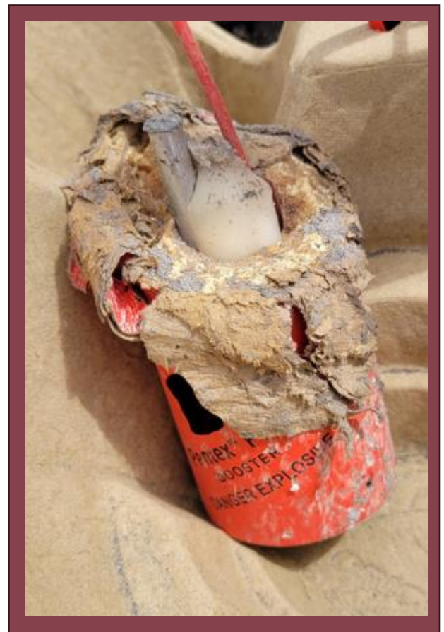
Figure 1 – Eroded booster with detonator
