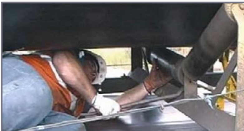
Figure 19: Awkward posture is required to access conveyor rollers. [9]
