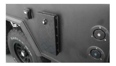
• **Ventilation Covers** – installation of aftermarket covers (to reduce dust and water ingress during offroad use) with no safety interlocks or provisions to ensure ventilation is uncovered when gas devices are in use.
